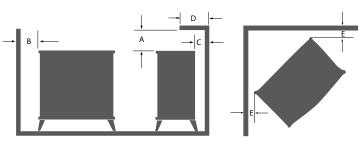
Minimum clearances to combustible materials in inches. Maintain clearance (empty space) between combustible materials and the heater as specified below for the appropriate model. Vermont Castings direct vent gas stoves must be installed on rigid flooring. When the heater is installed directly on any combustible surface other than wood flooring, a metal or wood panel extending the full width and depth of the unit must be used as the hearth.
