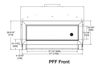
The PFF decorative front has an installed depth of 3/4" [19mm], measured from the front of the non-combustible finishing material to the front of the decorative front.
